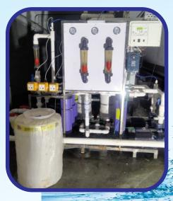
Flow of water through pipe may be measured with the help of Flow Meter and Rota Meter.
